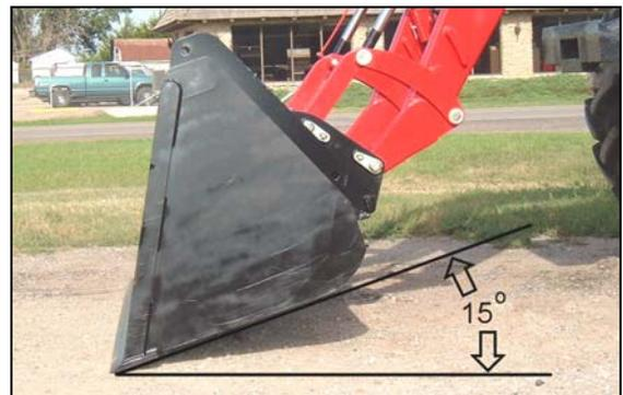
Never use bucket or other attachment in position shown to push or doze material. This will cause excessive pressure in bucket cylinder and will cause failure to your loader, which is not covered under warranty.
