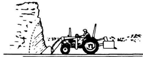
Side cutting is a good technique for cutting down a big pile.
