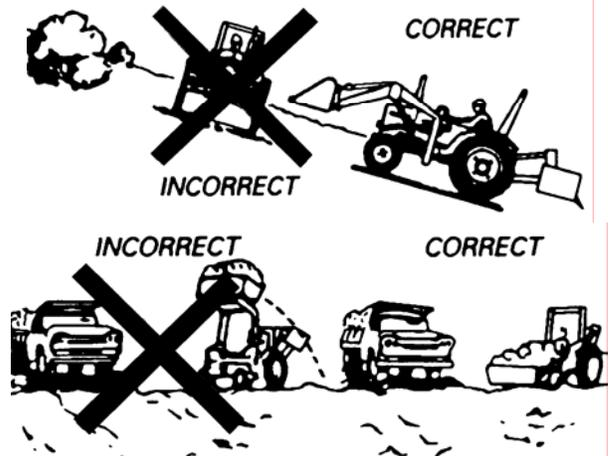
When transporting a load, keep the bucket as low as possible to avoid tipping, in case a wheel drops in a rut.
