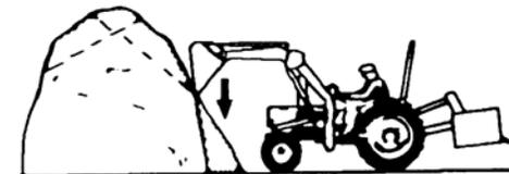
Another method for large dirt piles is to build a ramp approach to the pile.
