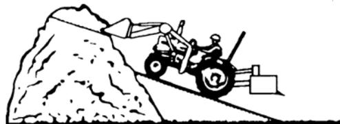
It is important to keep the bucket level when approaching a bank or pile. This will help avoid gouging the work area.
