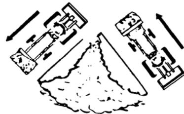
If the pile sides are too high and liable to cause cave-in, use the loader to break down the sides until a slot can be cut over the top.
