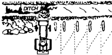
Pile dirt on the high side for easier backfilling on a slope.
